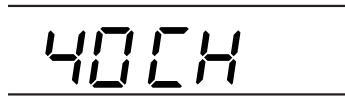
During Auto Channel Set The channel numbers are displayed as they are scanned and set.
